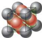
Face-centered cubic structure
