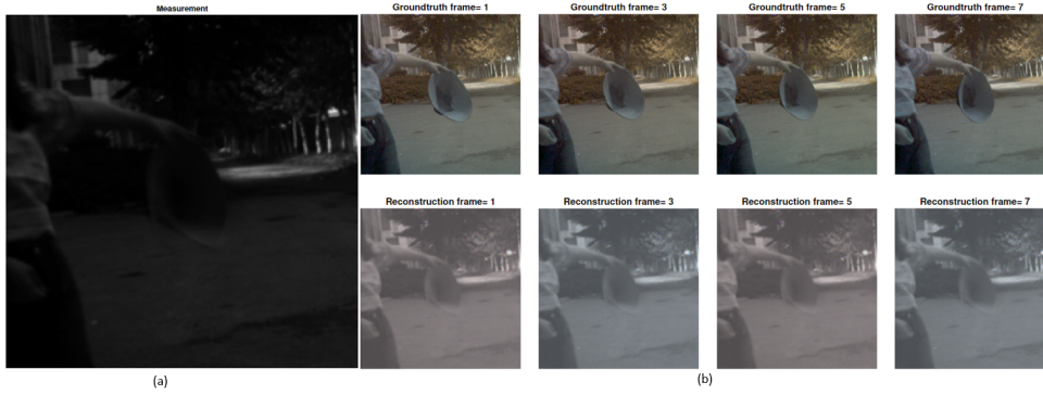
Fig. 1: Compressive measurement and comparison of image reconstruction quality. (a) Compressive measurement, (b) the first row shows 4 groundtruth frames. The second row depicts the recovered image using interpolation.
